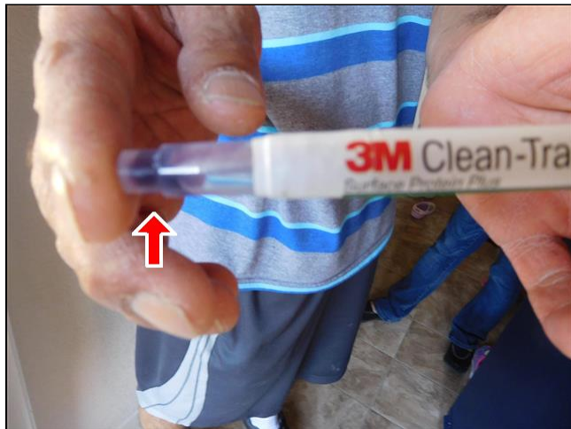
3.1 Item 1(Picture) Confirmed mold protein test at lower stair closet.
